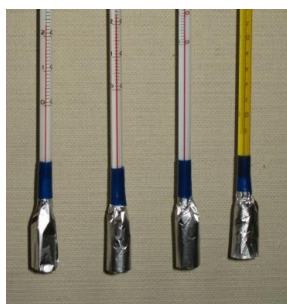
Photo 3 Mercury/ alcohol thermometers with radiation shields
