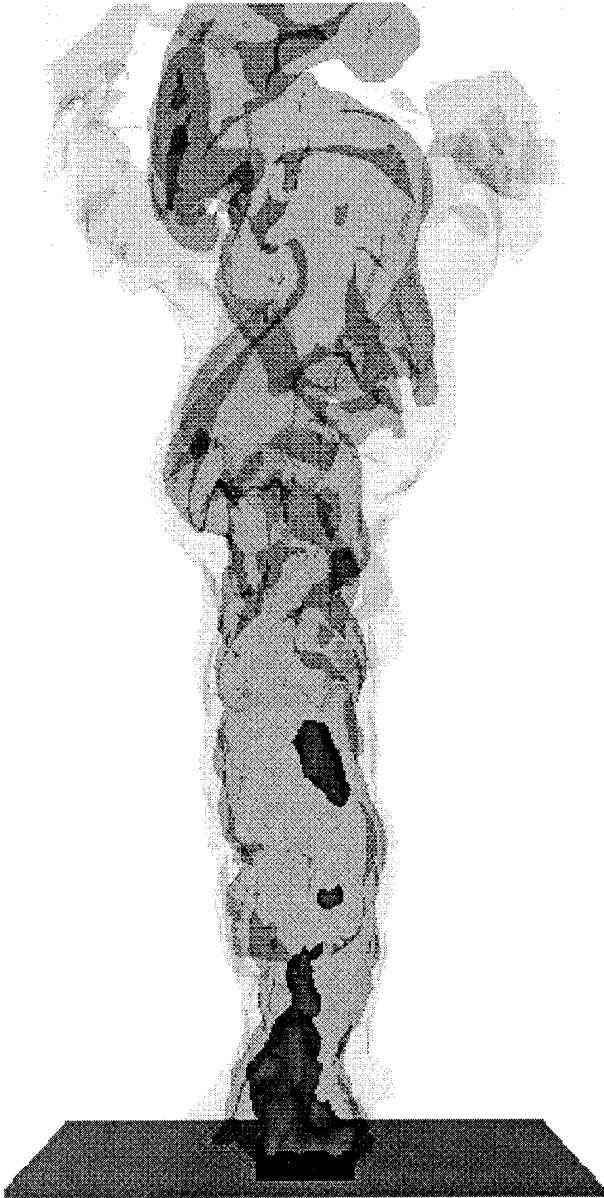
FIGURE 1: Instantaneous snapshot of a pool fire calculation performed on a 96 \times 96 \times 96 grid. The contours correspond roughly to the boundaries of the continuous flame, intermittent region and plume. The square burner is length D^* on each side, with the height of the domain rising about 12D^* .
